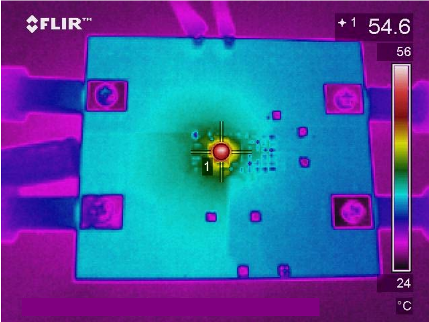
Fig. 13: Thermal Image of Top side of the board at 6A load Test points 1 is IR3856W
