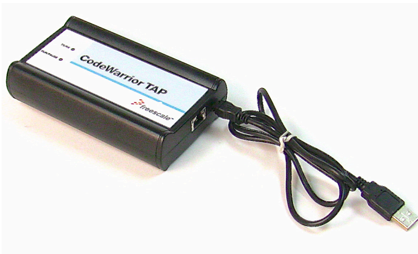
Figure 2.3 CodeWarrior TAP Probe with USB Cable Attached
