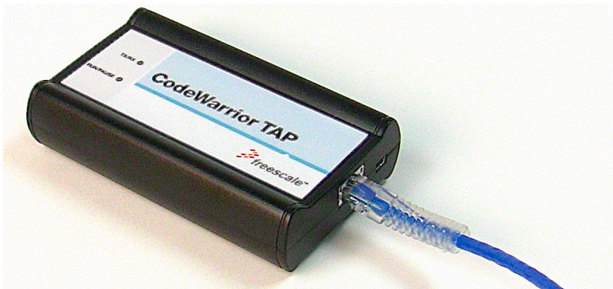
Figure 2.2 CodeWarrior TAP Probe with an RJ-45 Cable Attached
