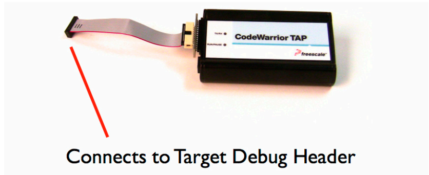
Figure 3.2 CW TAP Probe — Connecting to the Target
