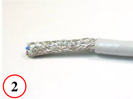
Strip off approx. 1" of cable jacket
