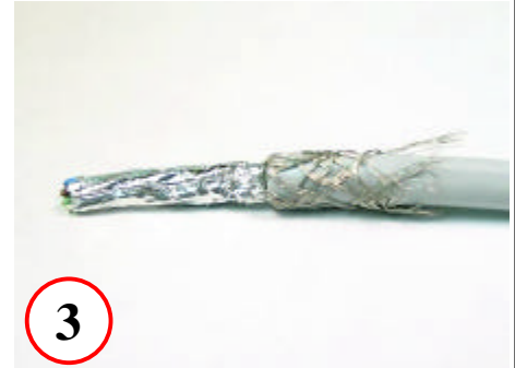
Fold outer shielding and drain wire back over cable jacket
